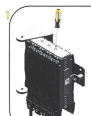
Put the CHT on front of the mounting kits. Insert 3 pcs M4 screws on each screw holes on top of the assembly.
