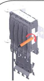
4.a To install the PEACOC® Clamshell Hardened Terminal (CHT), unscrew the captive screw using a wrench and rotate the unit clockwise to access the back portion.
