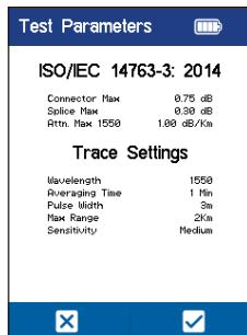
If the settings are correct, select the check box to start the test. A scanning status bar will be displayed, followed by a finding event message.
