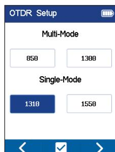
Select one or both wavelengths in either multimode or single-mode.
