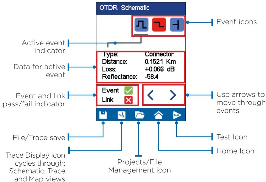
**OTDR Trace Screen** use Trace Display icon to cycle to the trace screen view.
