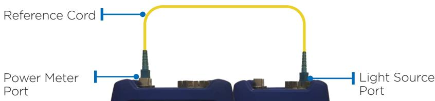
Touch reference indicator in the bottom right of the display and select, Set Reference to zero out the reference cord.
