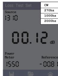
Touch the Modulation indicator to open the modulation options and set the modulation to CW for continuous wave.
