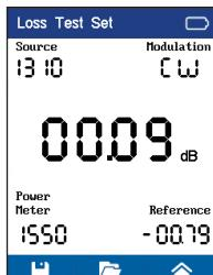
The value in dB, in the center of the display is the loss of the cable under test.
