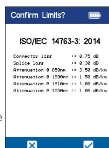
If a standard set of limits is selected, when the check box at the bottom of the display is touched, a page confirming those standards will be shown, such as this sample page.
