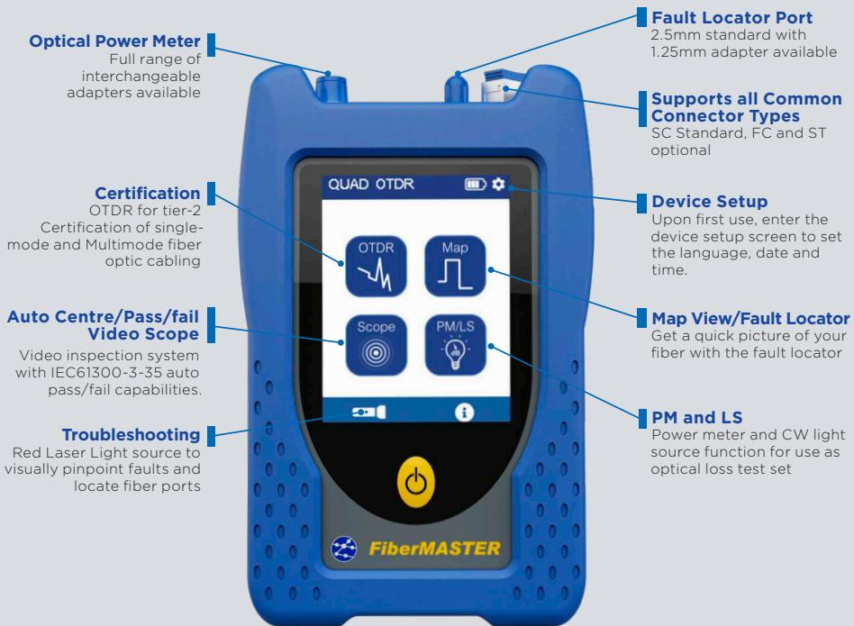
The TREND FiberMASTER range provides powerful performance in a small package. A simplified user interface is easy for beginners yet has full manual and custom setups for experienced users.
