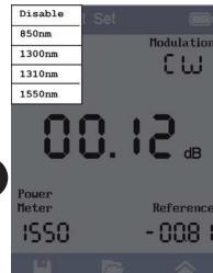
Touch the Source indicator to show the light source wavelengths available and select the desired wavelength for the test. Allow the light source 2-3 minutes to warm up and stabilize.
