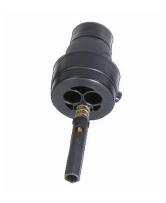
FIST Gel Sealing Kit for round splice closure port, sealing 2 cables with diameter between 8 and 11 mm
