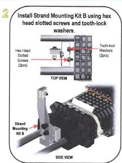
Insert the strand wire/cable on the D-Clamp teeth. Fasten the hex nut using wrench.
