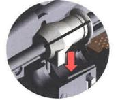
Use appropriate grommet for the type of cable being used.
