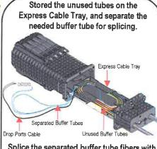
Splice the separated buffer tube fibers with the drop ports fibers. Store the fibers in the Splice Tray after splicing.
