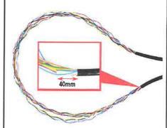
Cut the central membrane. Leave 40mm of the membrane from both ends of the jacket. Loosen the six (6) screws on Main Body and slide down the Cable Assembly Top & Bottom.
