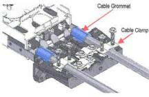
Put back the Cable Assembly Top and tightened the three (3) screws
