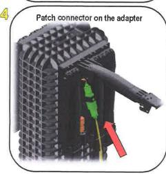
NOTE: Before patching the connector to the adapter, clean the end of the drop according to
