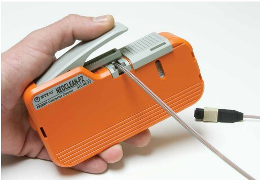
Cleaning PRIZM® LightTurn® connector
